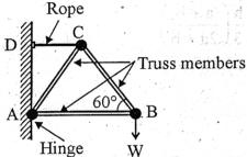
A three-member light weight plane truss ABC (with AB=BC) as shown in the figure is supported against a vertical wall by a horizontal rope CD. The force in the member AC will be
