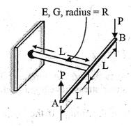
A rigid horizontal thin strip of length 2L is fixed at the free end of a circular cantilever of radius R and length L as shown in the figure. Vertical forces of magnitudes P are applied at the ends of the strip as shown. The modulus of elasticity and rigidity of the material of the cantilever are E and G respectively. The vertical deflection at point A due to the load is
