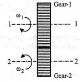
Power is transmitted from one shaft to a parallel shaft by a pair of external spur gears. If  $I_1$  be the mass moment of inertia of gear-1 about its own axis and  $I_2$  be the same for gear-2 then equivalent moment of inertia of the gearing system referred to the axis of gear-1 is
