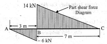
The part of the shear force diagram for a beam is shown in the figure. If the bending moment at B is – 9 kN.m, then bending moment at C is
