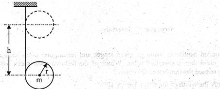
A chord is wrapped around a cylinder of radius r and mass m. If the cylinder is released from rest, the velocity of the centre of the cylinder after it has moved through a vertical and Improved and the matter tall in distance of h will be
